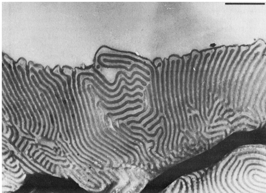
FIGURE 16 Electron micrographs of SI diblock copolymer ( MW = 524,000 g/mol, 52% styrene) at a free surface. (a) Lamellae oriented parallel to surface. (b) Lamellae oriented perpendicular to surface.
