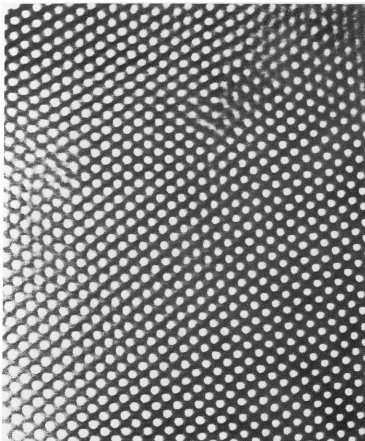
FIGURE 4 Transmission electron photomicrograph of an ultrathin film of a styrene-isoprene-styrene triblock copolymer (MW 16,200–75,600–16,200). \times 100,000 .
