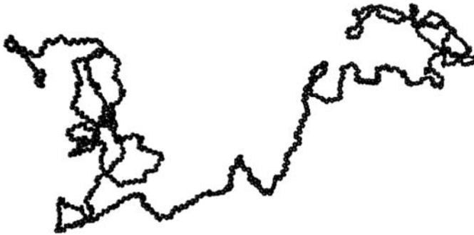
Figure 23.1 Snapshot of one isolated united atom model of PE ( N = 1000 ) obtained from molecular dynamics simulation after 10 ns equilibration at temperature 400 K
